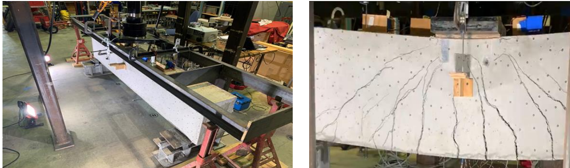
Figure 2. RC beam test setup (left) and the RC beam at the end of the test.
